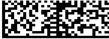
Figure 10 – The above are examples of both square and rectangular formats of the GS1 DataMatrix printed dark on light.
